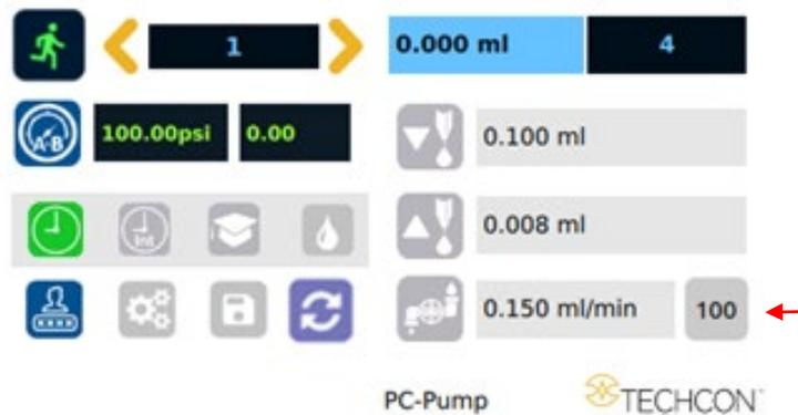
2. Enter desired flow rate (Note: Do not exceed recommended flow rate listed in the specification table).
