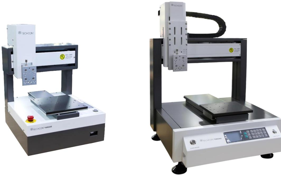
**Note:** the illustration may have some differences with each application. The dispensing equipment, such as a dispensing valve, syringe, cartridge, etc. are optional.
