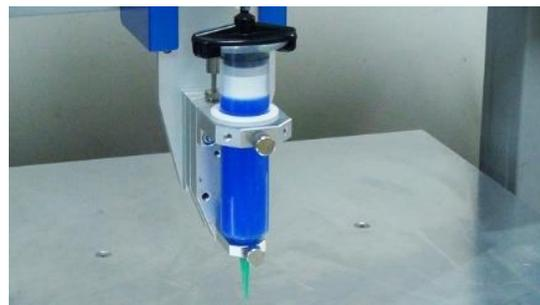
6. Install syringe and lightly tighten thumb screws.
