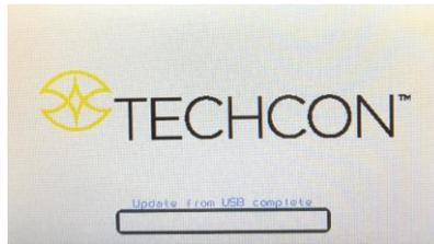
6. Wait until the system completes the software update from the USB drive and the first touch-screen calibration is displayed
