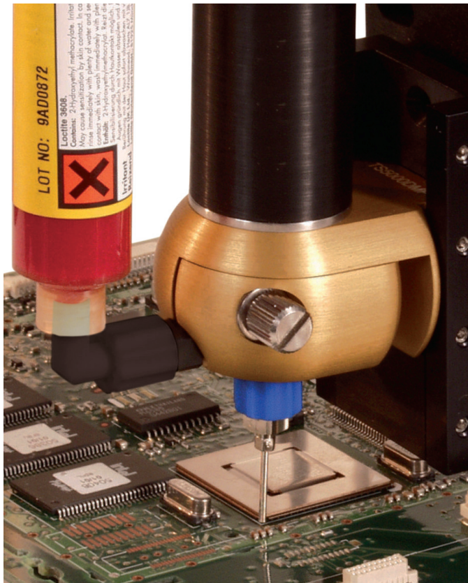
TS5000DMP - Performing underfill
