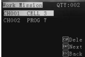
1 – Operation – Select the saved program, apply home adjust, process file, delete file, activate robot by external source (shortcut), setting purge and usage times.
