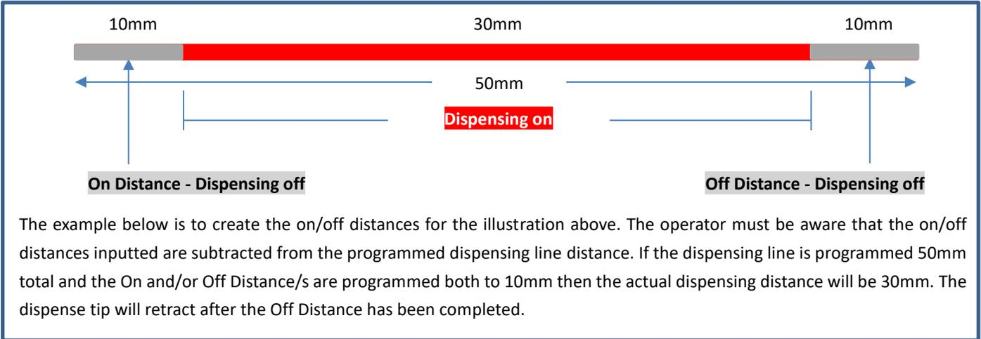
The example below is to create the on/off distances for the illustration above. The operator must be aware that the on/off distances inputted are subtracted from the programmed dispensing line distance. If the dispensing line is programmed 50mm total and the On and/or Off Distance/s are programmed both to 10mm then the actual dispensing distance will be 30mm. The dispense tip will retract after the Off Distance has been completed.
