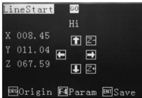
After selecting the type of dispensing (dot, line, arc...) use the jog keys to move to the Line Start position.
