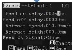
Set Feed on delay (dispensing time) Set retract height and speed.
