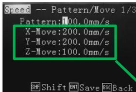
A change to the "Pattern" will apply this speed to all lines, polylines, circle and arcs, contained within the program. Individual speed changes can be changed by editing the program and selecting the co-ordinate (Line 1, Line 2), to edit.
