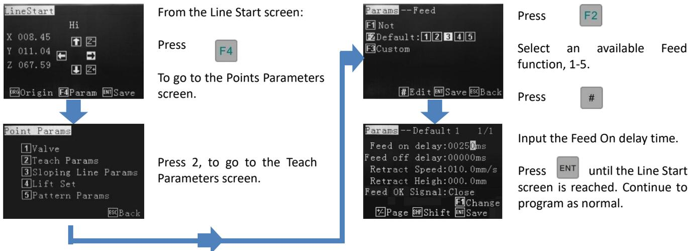
Up to 5 Feed On delay or 5 Feed Off delay times can be set per program. **Valve Feed Off Delay** is the time the robot will stay at the end of the dispensing location before moving to the next dispensing position. No fluid will be dispensed during to the Feed Off time period. Note that dots use a feed slot and could conflict will line start delay if the same slot is chosen for a dot and a line.
