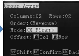
Input number of rows and columns. Order cannot be changed. Set "Mode" – dispensing direction. Press either **F1** or **F2**
