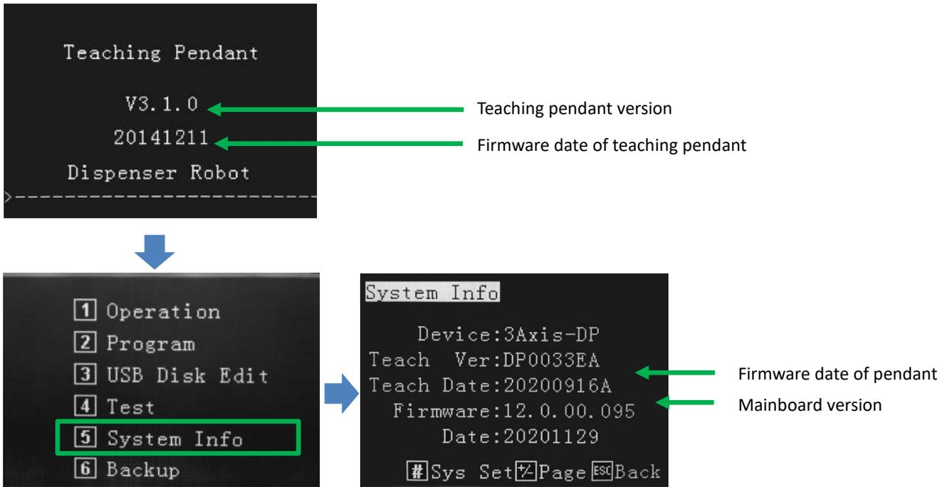
On the main robot front screen, whilst the teaching pendant is attached, the following information is displayed:
