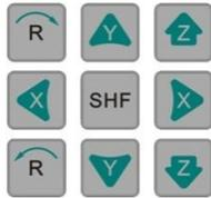
The TSR2000 Series robot is designed to be programmed by either inputting co-ordinates (advanced user) or by using the jog keys (entry level user).
