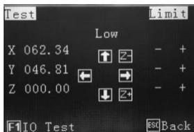
4 – Test – For testing areas of the robot such as axis jogging and I/O ports.
