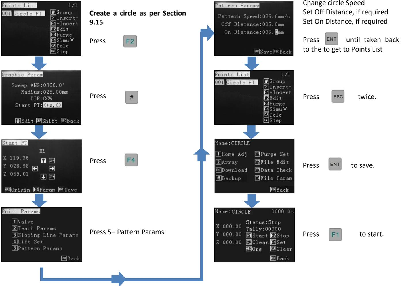
**Note:** If the pattern is 50mm in length and a 5mm On and Off Distance is set, the actual pattern will be 40mm (**50mm – 5mm On – 5mm Off = 40mm**). On/Off Distances should be added to the pattern length during programming or during editing.
