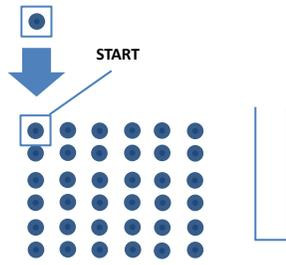
6 x 6 array to be created from a single dot element, showing start position and “Y” travel direction.
