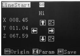
After selecting the type of dispensing (dot, line, arc...) input the X co-ordinate, using the number keys. Use the arrow keys to move down and input the Y and Z co-ordinates. When all 3 co-ordinates have been entered, press
