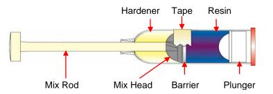
**INJECTION KIT**: For compound with a volumetric ratio of 10 parts or less per 100. The hardener is contained inside the valve mix rod while the resin is in the cartridge.
