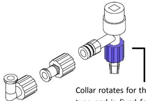
Collar rotates for the “R” type and is fixed for the standard type.
